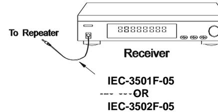
1. IR emitter (flat side) attached directly to IR sensor window
