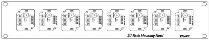
When using multi amplifier 8 pcs to fit in TPN008 rack, recommend to use attached jumper cable to extend power by one power adapter. (Recommend use DC12V 1.5Amp power adapter to support 8 pieces CA101HD)
