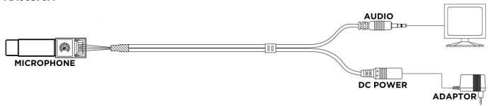
Remark: Since Hi sensitivity microphone, AA003PJA audio pick up box must be put at 5 meters away from monitor to avoid any audio reverberation.
