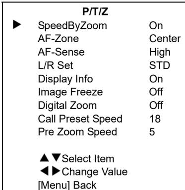
SpeedByZoom: The depth of field scale switch, optional items: On, Off.
