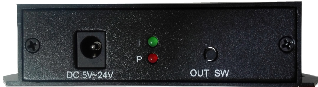
Power Input x 1 / Signal Indicator (Green) / Power Indicator (Red) / Output Switch Button
