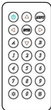
5.1 To command the matrix locally, setup the remote control IR01 ID with the same code of the Matrix (see 4.2). The default code is 0. (Power+0)
