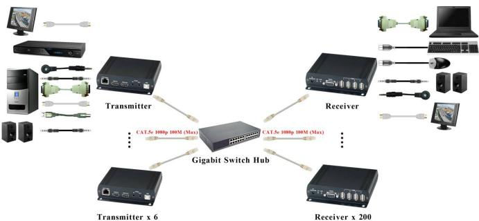
Multiple Inputs to Multiple outputs connections via a Gigabit network switch
