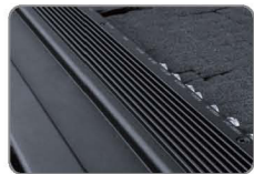
Video/audio controller heat discharge wings.
