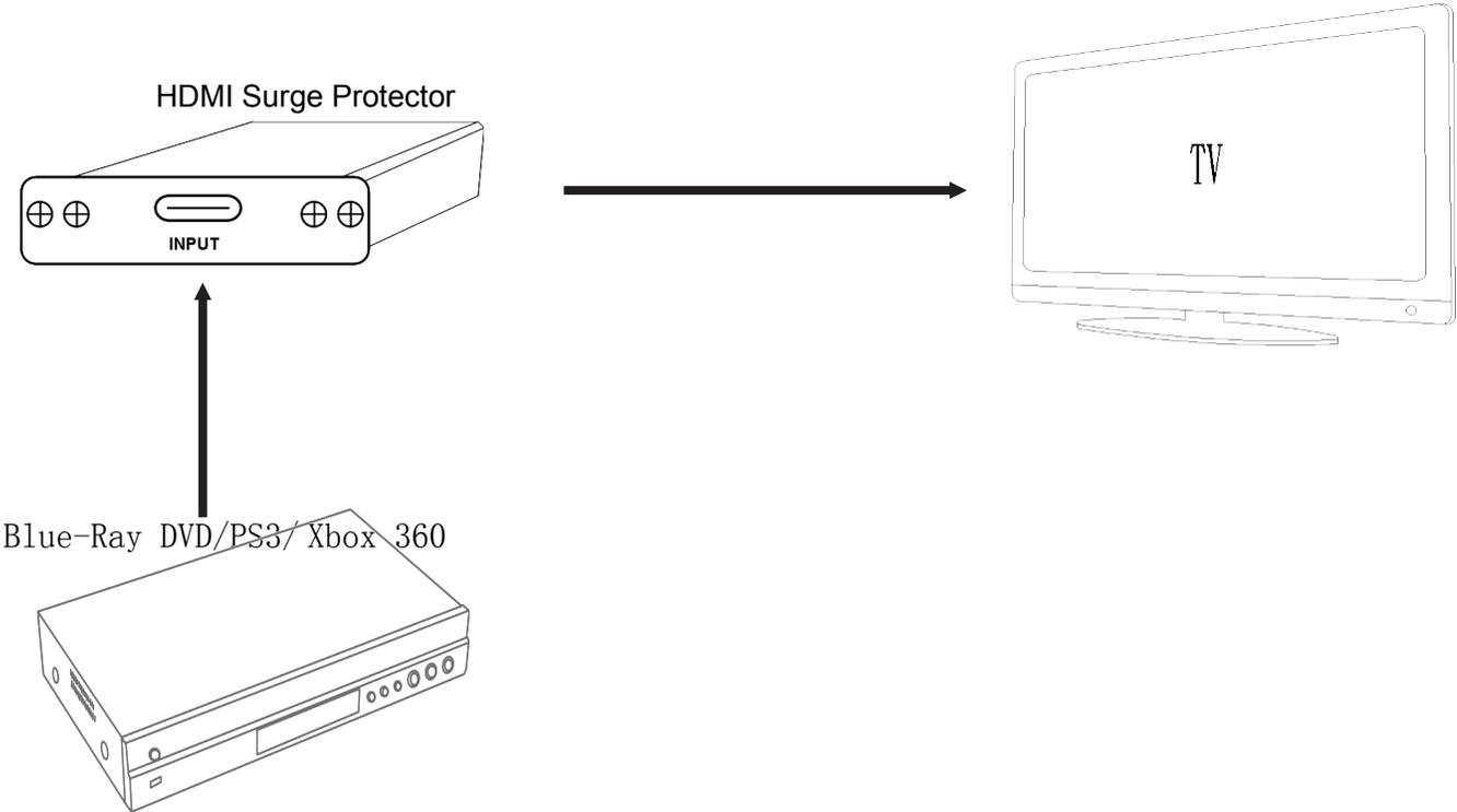
1. To connect the HD Source with the HDMI input port of the HDMI surge protector
