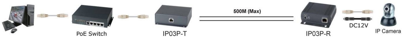
IP03PT with POE switch power input to IP03R and Non-POE IP camera.
