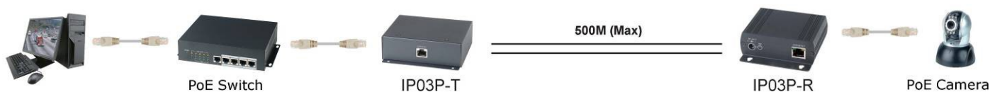
IP03PT with POE switch power input to IP03R and POE camera
