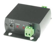
The RS001R is designed to extend the RS485 beyond the 1200 meters limitation, or whenever there is a need to "boost" the RS485 signal. It could works 32 multi-drop RS-485 LAN configuration. In a half-duplex multi-drop environment all RS-485 nodes share the same data lines. A single pair of data lines act as both transmit and receive wires.
