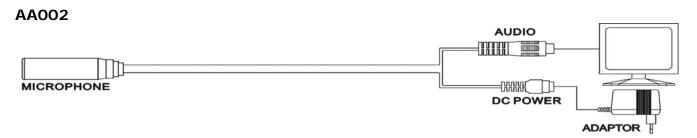
Remark: Since Hi sensitivity microphone, AA001/AA002 audio pick up box must be put at 5 meters away from monitor to avoid any audio reverberation.
