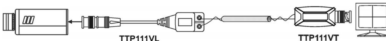
\* Used as a transmitter, the TTP111VL Weather Proof IP65, has a 25cm Mini coax cable to be suitable install with outdoor camera.
