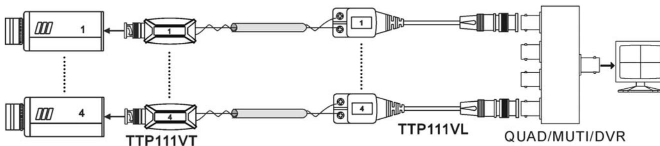
\* Used as Receiver, the TTP111VL compact size is perfect to connect with the image processor, which have multi BNC connections, as like Multiplexer, Quad, DVR ...etc.
