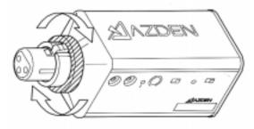
To plug the 41XT onto a microphone (low impeadance with XRL connector) first make certain the the locking-ring is turned fully up (rotate counter-clockwise). Then plug the 41XT fully into the microphones XLR connector and tighen by rotating the ring fully down (clockwise).
