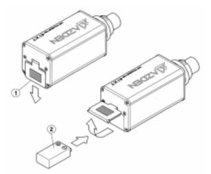
**41XT** plug-in XLR transmitter with 63 on-board user selectable UHF frequencies. Ideal for use with dynamic microphones with XLR output.
