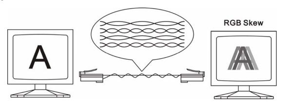
2. Recommend to use following cabling way to reduce skew status, to add special made "skew immunized adaptor", 2 pieces included at the package.
