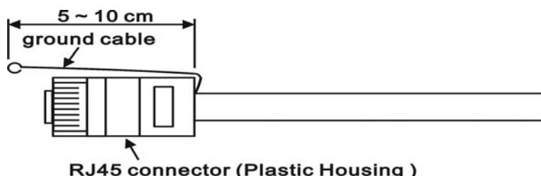
2. Make the ground cable connect to ground screw, then plug RJ45 connector.
