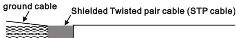
2. STP (shielding) RJ45 connector with STP cable connection.
