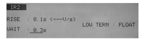
In DC insulation resistance testing, if a test voltage is applied to a DUT that contains capacitive elements, the measured insulation resistance will be below the optimal value due to a charge current, until charging is completed. To avoid upper fail judgment by the charge current, a wait time must be provided from the starts of START VOLTAGE, and upper fail judgment will be ignored during wait time.
