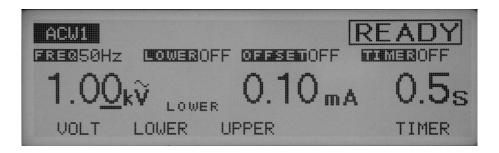
To make a setting, use the rotary knob with the cursor at the test voltage.
