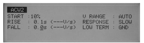
When the test ends with a PASS judgment, the voltage falls to 0 V during the preset voltage fall time. This voltage fall time can be set to 0.0 s through 200 s (at a resolution of 0.1 s for the 0.1 s to 99.9s range and 1 s for the 100 s to 200s range).
