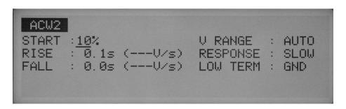
For an AC withstanding voltage test, set the start voltage as a percentage of the test voltage, to 0% through 99% (at a resolution of 1%). When the cursor is located to the right of START, settings can be made using the rotary knob.
