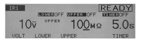
The upper resistance can be set to 0.01 M $\Omega$  through 9.99 G $\Omega$  (at a resolution of 0.01 M $\Omega$  for the 0.01~9.99 M $\Omega$  range, 0.1M $\Omega$  for the 10.0 M $\Omega$  to 99.9 M $\Omega$  range, 1M $\Omega$  for the 100M $\Omega$  to 999M $\Omega$  range, and 0.01G $\Omega$  for the 1.00G $\Omega$  to 99.9G $\Omega$  range), but below the maximum rated current.
