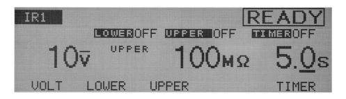
The time during which a preset voltage is applied to the DUT can be set to between 0.5 s and 999 s (at a resolution of 0.1 s for the 0.5 s to 99.9 s range and 1 s for the 100 s to 999 s range).
