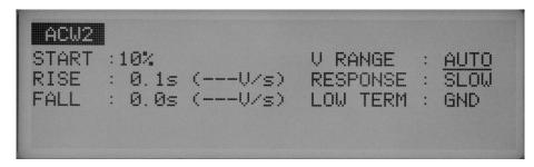
Switch the output-voltage ranges. For the output-voltage range, select between AUTO and 5kV. The 5kV range can be changed at any time up to 5.20kV. the AUTO range automatically selects either the 2.5kV range or the 5kV range, as it is selected in the pre-test settings. If the pre-test setting exceeds 2.6kV, the 5kV range is selected. Otherwise, the 2.5kV range is selected. Once the 2.5kV range has been selected, the voltage cannot be reset above 2.6kV during the test.
