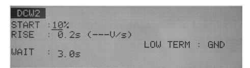
For a DC withstanding voltage test, set the start voltage as a percentage of the test voltage, to 0% through 99% (at a resolution of 1%). When the cursor is located to the right of START, settings can be made using the rotary knob.
