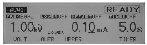
The lower current can be set between 0.01 mA and 110 mA (at a resolution of 0.01 mA for 0.01 mA to 9.99 mA, 0.1 mA for 10.0 mA to 99.9 mA, and 1 mA for 100 mA to 110 mA). When the cursor is at the lower current, the rotary knob can be used to make settings. When the lower judgment function is set to ON and the measured current is at or below the lower current, the test ends with a FAIL judgment.
