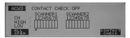
When the optional high-voltage scanner TH9121 (with a contact check function) is connected to the tester, the continuity between the test lead wire and the DUT can be checked using the HIGH or LOW terminal prior to the application of a test voltage.
