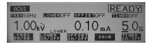
The frequency of the test voltage can be set to either 50 Hz or 60 Hz. The test frequency can be set using the SHIFT + F1 keys (press the F1 key while pressing the SHIFT key), regardless of where the cursor is positioned. Every time the SHIFT + F1 keys are pressed, the setting alternates between 50 Hz and 60 Hz.
