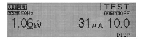
(••) The tester saves the offset value that is valid when the STOP-switch is pressed or the preset timer time has elapsed. Upon completion of the offset measurement, the tester returns to the READY status.
