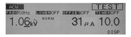
The time is displayed differently depending on whether the timer function is on or off. The timer is ON : The remaining test time is displayed.
