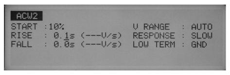
The rise time between the start voltage and the test voltage can be set to 0.1 s through 200 s (at a resolution of 0.1 s for the 0.1 s to 99.9s range and 1 s for the 100 s to 200s range).
