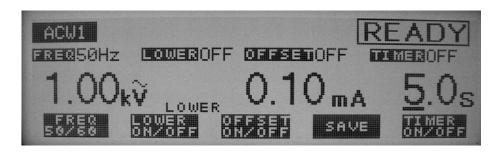
The lower judgment function can be turned on/off. When the lower judgment function is on, the test result is judged to be FAIL if the measured current drops below the lower current, and the test is ended.
