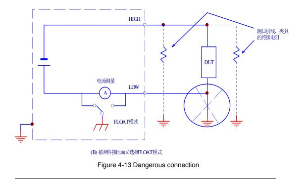
Select FLOAT only when DUTs such as small electronic components and jigs are completely "floating" electrically.
