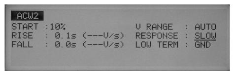
By changing the integrated time constant of the current detection circuit, switch the current detection response for UPPER FAIL judgment.
