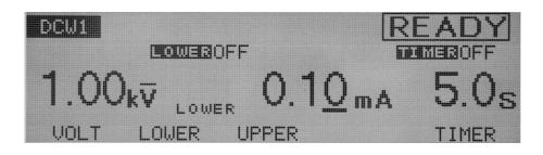
The lower current can be set between 0.01 mA and 11.0 mA (at a resolution of 0.01 mA for the 0.01 mA to 9.99 mA range, and 0.1 mA for the 10.0 mA to 11.0 mA range).
