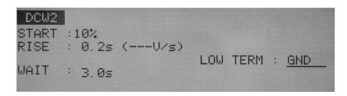
You can select either of the following two measurement modes; The **GND** mode that the LOWTERM is connected to the tester's LOW terminal, The **FLOAT** mode that the LOWTERM is used as guard. In both modes, the tester detects the current flowing into the LOW terminal from the HIGH VOLTAGE terminal via the DUT.
