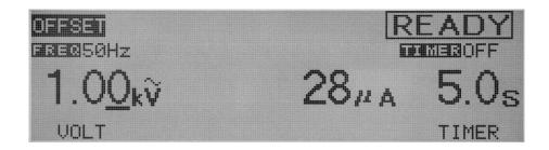
4. When necessary, set the test voltage, test frequency, and test time. For the setting procedures.
