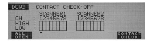
When the optional high-voltage scanner TH9121 (with a contact check function) is connected to the tester, the continuity between the test lead wire and the DUT can be checked using the HIGH or LOW terminal prior to the application of a test voltage.
