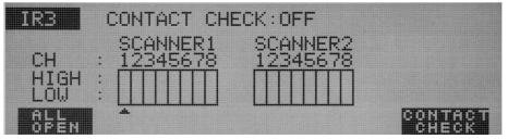
When the optional high-voltage scanner TH9121 (with the contact check function) is connected to the tester, the continuity between the test lead wire and the DUT with the HIGH or LOW terminal can be checked prior to the application of a test voltage. To do so, turn on the contact check function.
