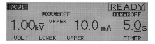
The time during which a preset voltage is applied to the DUT can be set to 0.3 s through 999 s (at a resolution of 0.1 s for the 0.3 s to 99.9s range and 1 s for the 100 s to 999s range). When the cursor is at the timer, the rotary knob can be used to make settings.
