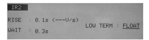
You can select either of the following two measurement modes; The **GND** mode that the LOWTERM is connected to the tester's LOW terminal, The **FLOAT** mode that the LOWTERM is used as guard.
