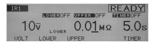
The lower resistance can be set to 0.01 M through 9.99 G (at a resolution of 0.01M for the 0.01-9.99 M range, 0.1 M for the 10.0 M to 99.9 M range, 1 M for the 100 M to 999 M range, and 0.01 G for the 1.00 G to 9.99 G range), but below the maximum rated current. When a resistance value at or below the lower resistance is detected following a wait time, the test ends with a FAIL judgment.
