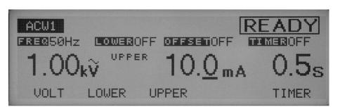
The upper current can be set between 0.01 mA and 110 mA (at a resolution of 0.01 mA for the 0.01 mA to 9.99 mA range, 0.1 mA for the 10.0 mA to 99.9 mA range, and 1 mA for the 100 mA to 110 mA range). When a current exceeding the upper current is detected, the test ends with a FAIL judgment. When the cursor is at the upper current, the rotary knob can be used to make settings.
