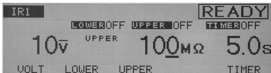
The upper resistance can be set to 0.01 MΩ through 9.99 GΩ (at a resolution of 0.01 MΩ for the 0.01~9.99 MΩ range, 0.1MΩ for the 10.0 MΩ to 99.9 MΩ range, 1MΩ for the 100MΩ to 999MΩ range, and 0.01GΩ for the 1.00GΩ to 99.9GΩ range), but below the maximum rated current.
