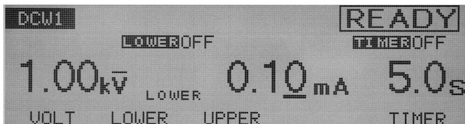
The lower current can be set between 0.01 mA and 11.0 mA (at a resolution of 0.01 mA for the 0.01 mA to 9.99 mA range, and 0.1 mA for the 10.0 mA to 11.0 mA range).
