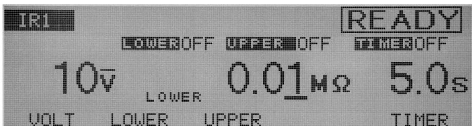
The lower resistance can be set to 0.01 M through 9.99 G (at a resolution of 0.01M for the 0.01-9.99 M range, 0.1 M for the 10.0 M to 99.9 M range, 1 M for the 100 M to 999 M range, and 0.01 G for the 1.00 G to 9.99 G range), but below the maximum rated current. When a resistance value at or below the lower resistance is detected following a wait time, the test ends with a FAIL judgment.
