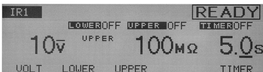
The time during which a preset voltage is applied to the DUT can be set to between 0.5 s and 999 s (at a resolution of 0.1 s for the 0.5 s to 99.9 s range and 1 s for the 100 s to 999 s range).
