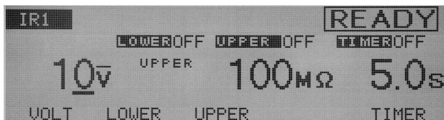
The test voltage to be applied to a DUT can be set to DC –10 V through –1020 V (at a resolution of 1 V). (The negative (-) mark is not displayed.)
