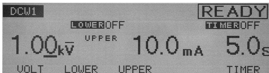
The test voltage to be applied to a DUT can be set to DC 0.00 kV through 6.10 kV (at a resolution of 0.01 kV).
