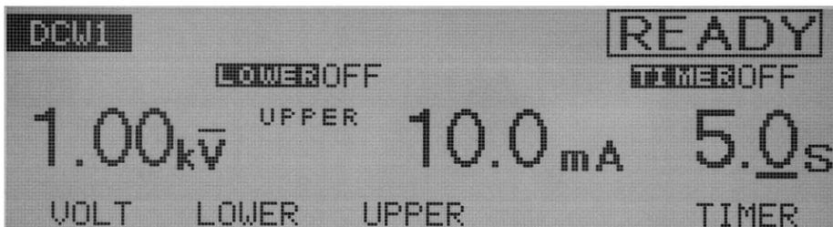
The time during which a preset voltage is applied to the DUT can be set to 0.3 s through 999 s (at a resolution of 0.1 s for the 0.3 s to 99.9s range and 1 s for the 100 s to 999s range).
