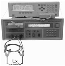
■ From the measuring impedance values above you will see if the instruments are connected and working normally. In general, short circuit impedance should be as low as possible and open circuit impedance should be as large as possible. The measuring results when bias current is disabled should be consistent with the results measured directly by a L/LCR meter.
