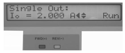
8) Press [F/R] key to change the current direction between FWD(+) and REV(-). When a reverse current is outputted, LED REV(-) will be lighted as shown in the following figure.
