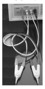
Short the test terminals as shown in the following figure to perform the SHORT correction for LCR meter.
