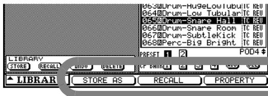
Figure 2.6: POD keys 2 through 4 used as soft keys
