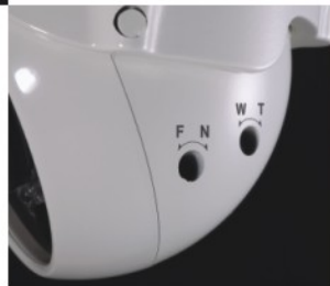
Waterproofing exterior adjustment vari-focal lens
