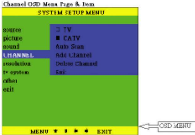
On channel Sub-menu, Select **TV** for receiving Terrestrial VHF/UHF broadcasting channel. Select **CATV** if the unit is connect to a CATV coaxial cable.
