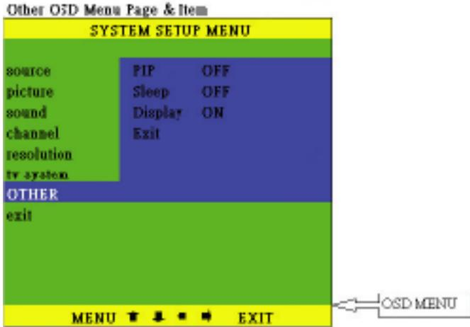
**Display:** Set " ON " to display the input/output information on the screen.
